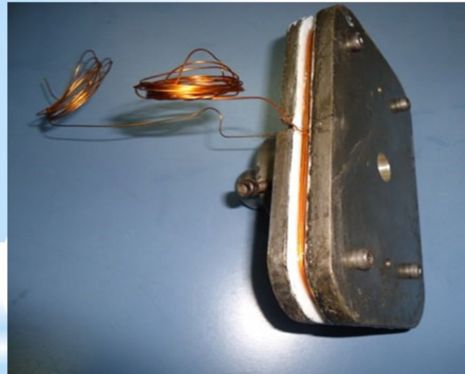
Core insulation with Kapton
