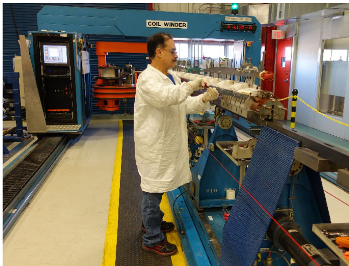
QXFA coil winding
