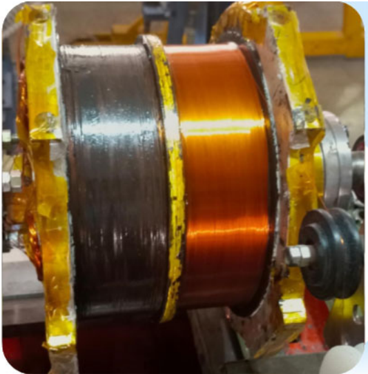
Bucking coil 2 first layer
