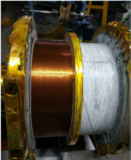
BC 1 winding first layer
