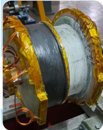
Bucking coil 1 last layer after STYCAST
